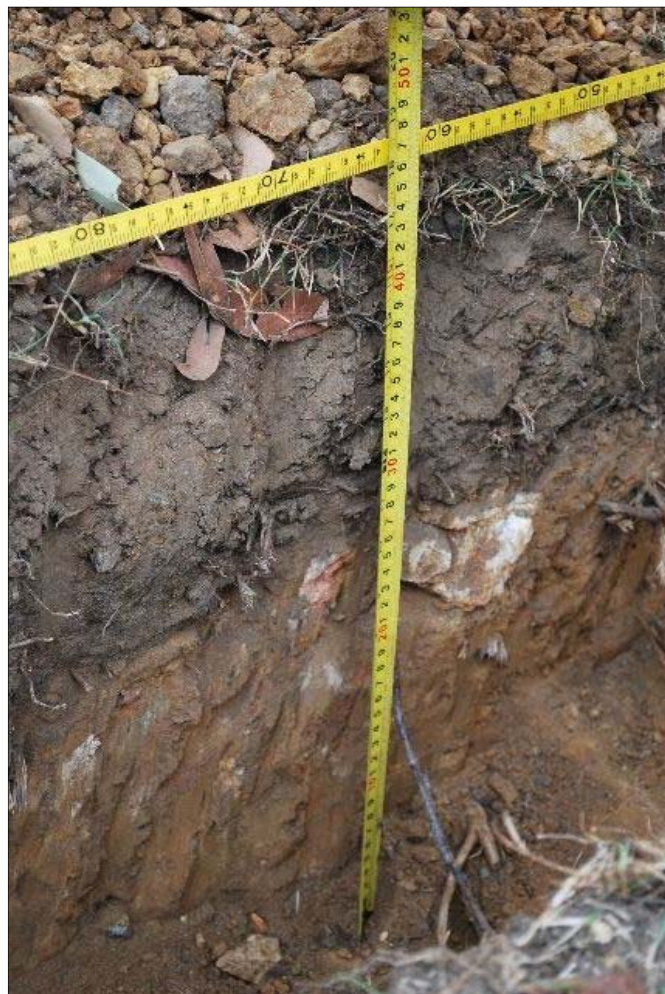
Trench depth to 500mm. The clearly visible lower soil horizon comprises of hard compacted clay sub soils containing large sand stone boulders.
