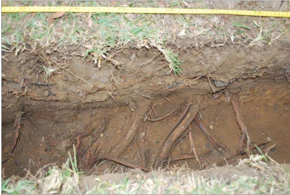
Roots located at 7.9m – 9.0m along trench. Low numbers of small diameter (<10mm) roots were also present in the trench.
